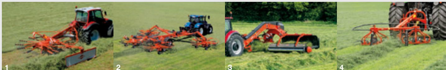
1. Mounted single-rotor - 2. Semi-mounted with 4 rotors - 3. Belt mergers - 4. Tedder-rakes
