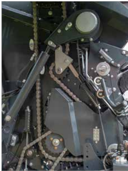
10. Robust driveline with wear-resistant and oversized chains
