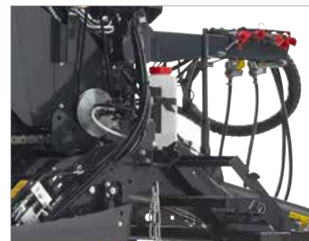
6. BEKA-MAX continuous chain oiling system
