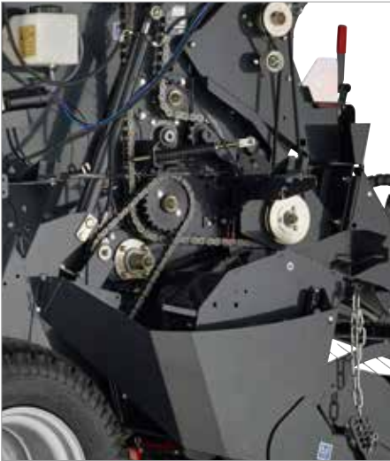
1. Robust driveline with high-quality IWIS chains
