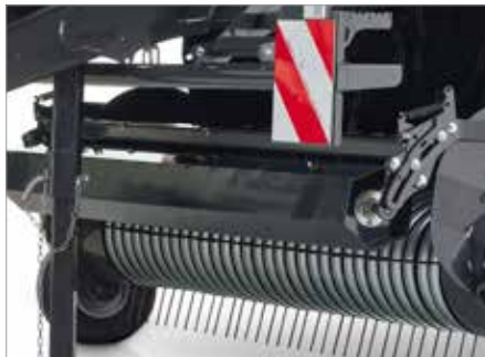
5. Spring-loaded crop tines and heavy crop roller (Ø 217 mm) for improved pre-compression and crop flow
