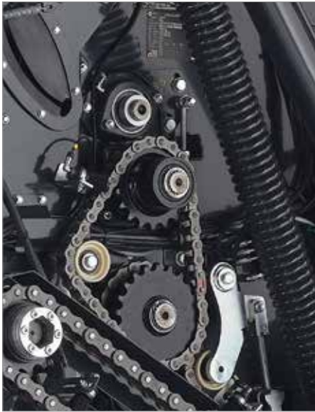
1. Second drive roller guarantees a secure belt drive in all crop conditions
