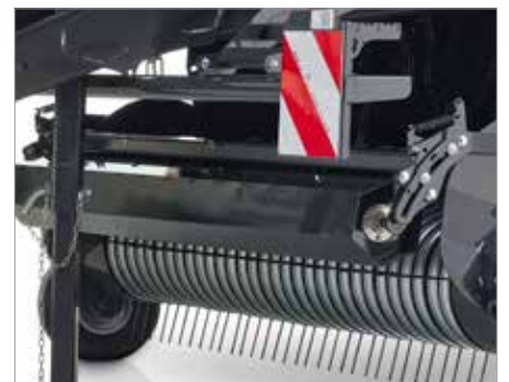
4. Spring-loaded crop tines and heavy crop roller (Ø 217 mm) for improved pre-compression and crop flow
