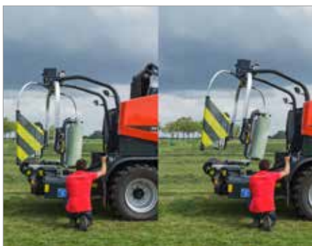
8. VBP 7190: Integrated wrapper adjustment to unload bales larger than 1.60 m
