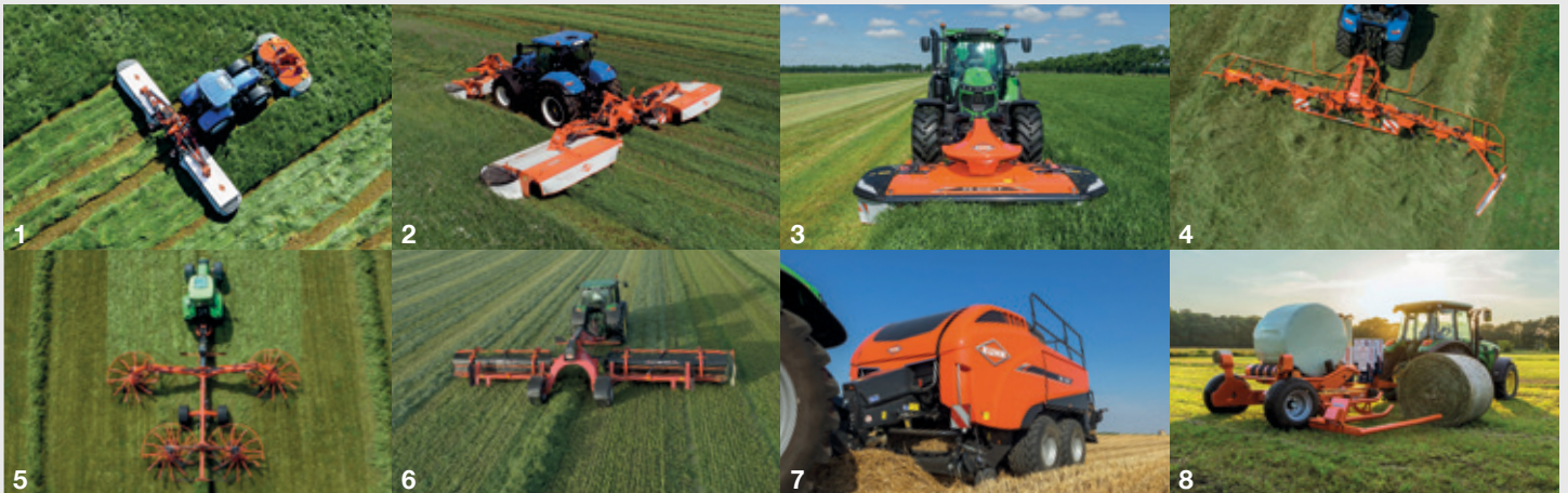
1. Disc mowers - 2. Disc mower conditioners - 3. Drum mowers - 4. Gyrotedders - 5. Gyrorakes - 6. Belt mergers - 7. Balers - 8. Wrappers
