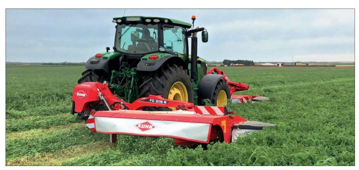
KUHN has combined conditioner, LIFT-CONTROL suspension and vertical folding, for the first time in one machine, to create the new FC 3115 D and FC 3115 R front-mounted mower conditioners. These new models of mower conditioners have a working width of 3.10m. They are designed for forage farms and contractors, and can be used with a front mower to increase work output.
