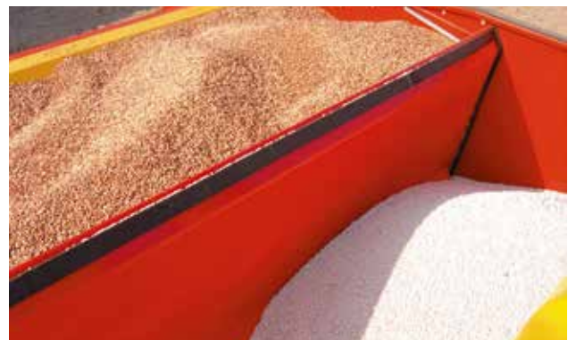
Rapid 300-400C/S has a high capacity hopper. On the combi models, the relation between seed and fertiliser is easily altered.
