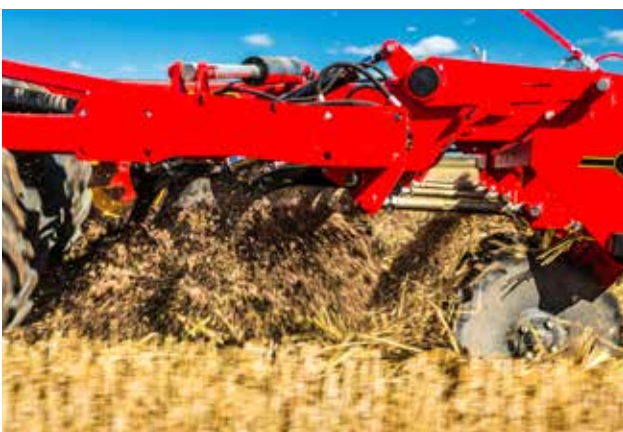
By performing multiple operations, TopDown is able to create a good seedbed in one pass.
