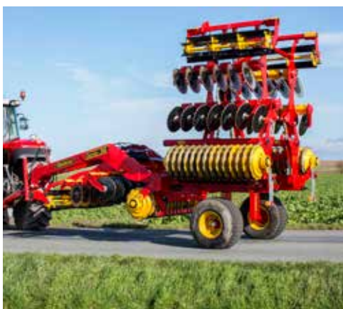
The unique folding gives Carrier 420-820 a low center of gravity and good manoeuvrability in transport, as well as excellent contour following in the field.
